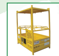
Personnel Basket 1350 x 1350 x 2420 Gross: 980kg Tare: 480kg Payload: 500kg
