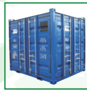
10'x8'x8'6" Dry Goods 2991 x 2438 x 2591 Gross: 10,000kg Tare: 2,010kg (Standard)/ 2,400kg (with Side Door) Payload: 7,990kg/7,600kg
