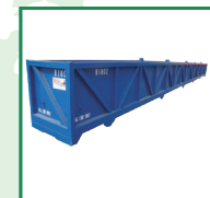
18.3m Cargo Basket 60' x 4' x 4'7" 18300 x 1200 x 1425 Gross: 16,500kg Tare: 5,350kg Payload: 11,150kg
