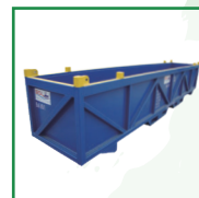
6.3m Cargo Basket 21' x 4' x 4'3" 6300 x 1200 x 1300 Gross: 13,000kg Tare: 1,900kg Payload: 11,100kg
